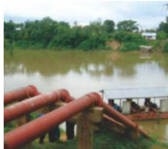
Lowland farms often pump water from nearby tributaries or wetlands. The water level of these sources changes significantly between the wet and dry seasons, as backwater flows up from tributaries and some places along the Mekong. A floating pump or 'pontoon' method is used to cope with these changes. Some farmers also used drip irrigation systems.
